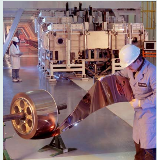
The Ovonic continuous web triple-junction machine manufactures photovoltaics continuously by the mile and by the ton.
